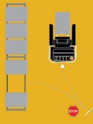
**180° steering.** Truck has to come to a stop and direction of travel selected manually by operator. **360° steering.** Drive wheel rotates 270° when maneuvering within the aisle without stopping.
